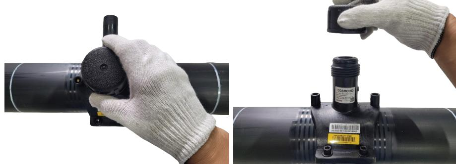
B. Insert tapping tool into punch.
