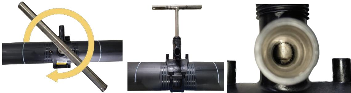
D. Punch upward by rotating counter-clockwise until the punch is level with the top of the fitting chimney. Do not remove punch from chimney.
