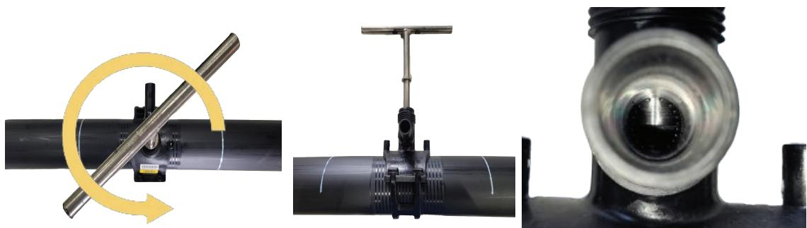
E. Remove the tapping tool. If necessary, lubricate the cap and chimney O-ring and replace the cap. Tighten cap hand tight only, do not use wrenches. Check for leaks per normal procedures.
