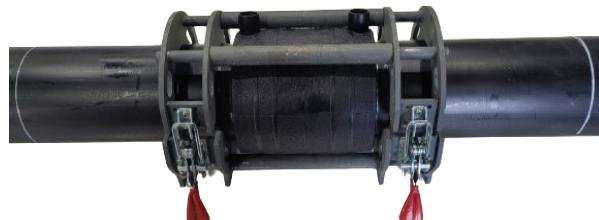
I. Connect the control box leads to the fitting, verify that the proper fusion time and voltage are displayed on the control box, and fuse the joint. Do not leave the fusion unattended.
