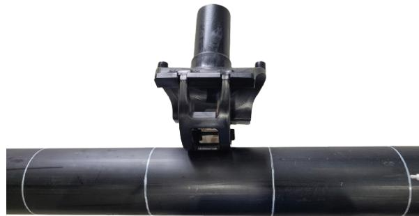
C. Scribe witness marks on the pipe surface, or mark the area to be scraped or peeled in a criss-cross pattern.
