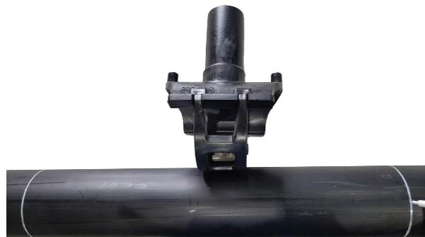
B. Mark slightly larger than the width of saddle to be installed. These marks indicate the scrape or peel length required to ensure that only scraped or peeled pipe touches the saddle fusion surface. It is recommended to scrape or peel slightly longer than required outside the fusion zone as visual evidence that proper preparation has been made.
